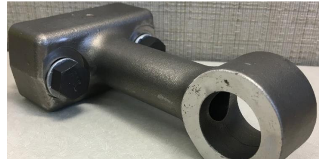
Image 2: Fuel Injection Pump Inlet Pipe (Banjo Fitting)
