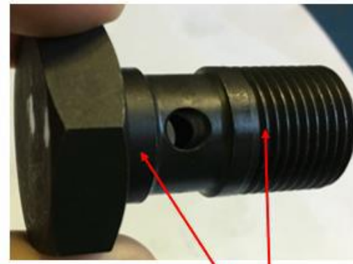
Image 3: Banjo Bolt showing radial through-hole and hollow shank. (Red arrows indicate where steel washers w/ O-ring fit.)
