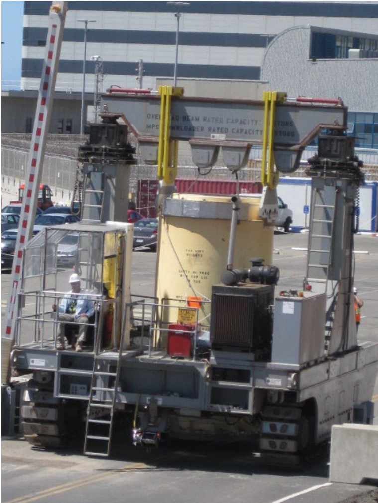
Transporting Loaded MPC in Transfer Cask to ISFSI
