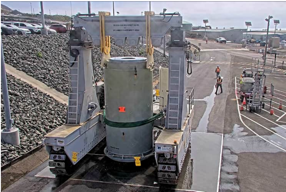
Transporting Loaded MPC in Transfer Cask to ISFSI
