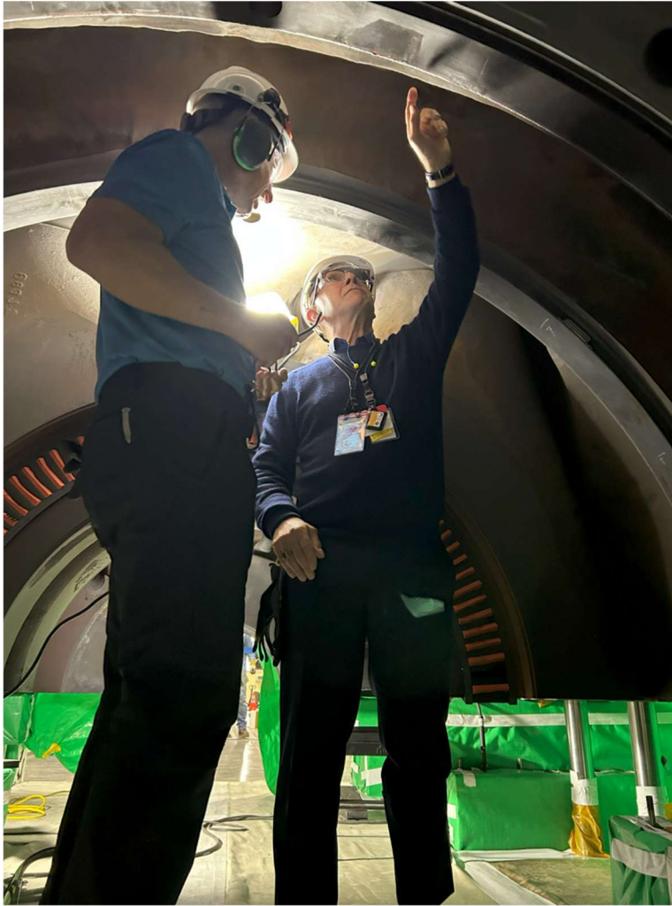
DCPP Technician and Dr. Meshkati Looking at Weld Repairs Under the HP Turbine Upper Casing
