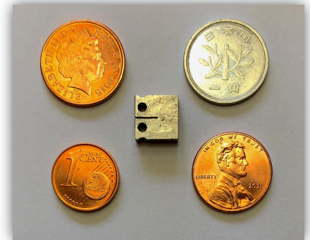
Mini-CT Fracture Toughness Specimen
